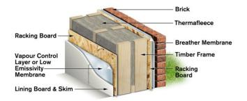
The twin frame system ensures that reduced thermal bridging occurs within the construction helping maximise insulation performance. By using two 89mm structural timber frames, the width of the construction can be varied to achieve specific insulation performance.
